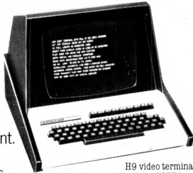
H9 video terminal, with 67 ASCII keys.
